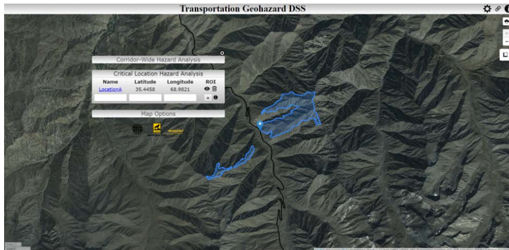
Figure 12. Hazard zone created on the fly for a user-defined point along the corridor.
